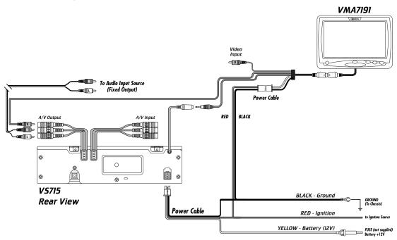
Figure 13. Wiring diagram for VS715.
